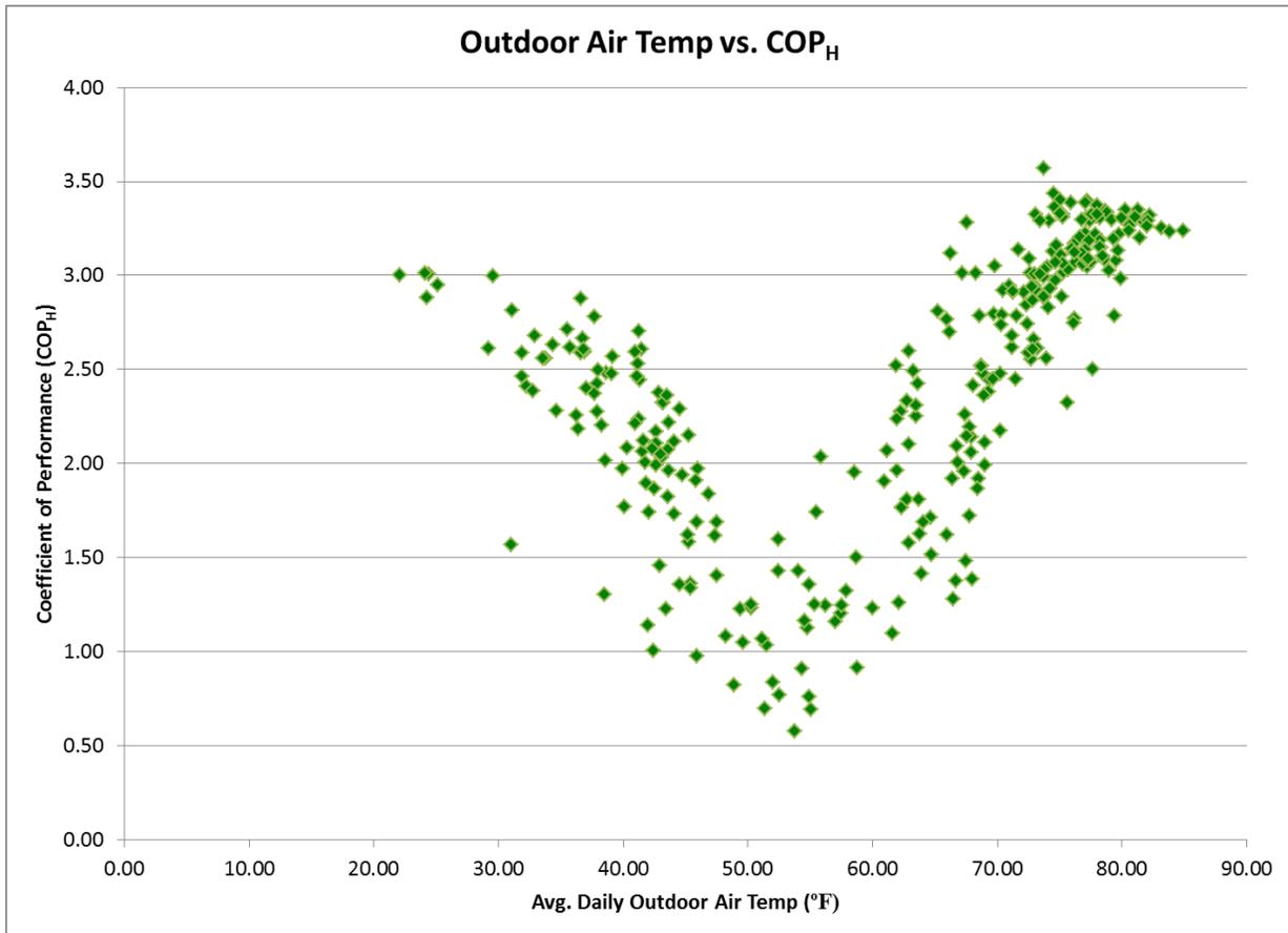
Figure 17. Geothermal system efficiency (COP<sub>H</sub>) compared directly to average daily outdoor air temperature (in degrees Fahrenheit).
