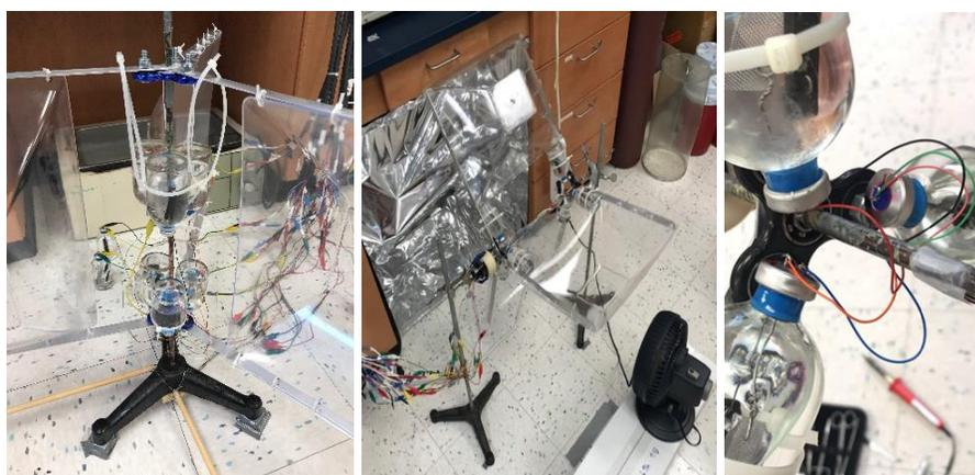
Figure 2A. The vertical WAVE digester is to the far left, and the horizontal WAVE digester is in the middle. The wires were soldered from the potentiostat onto the anode and cathode of each reactor so the proper voltage for each respective reactor could be applied.
