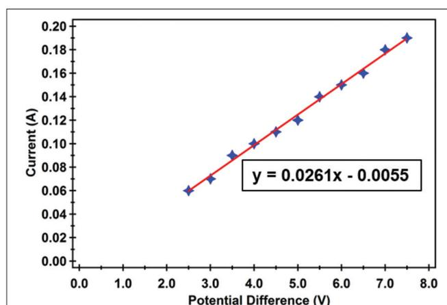
Fig. 1. Plot of current vs. voltage for an ADDA model fan. After a linear fit of the data, the fan's effective resistance can be taken as the reciprocal of the slope. From this data set, the effective resistance of the fan was found to be  $38.3 \Omega$ .
