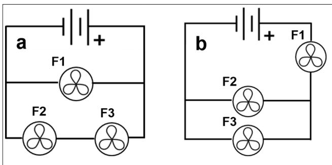
Fig. 2. Circuit diagrams for the combination circuits with (a) two fans in series with one in parallel and (b) two fans in parallel with one in series.
