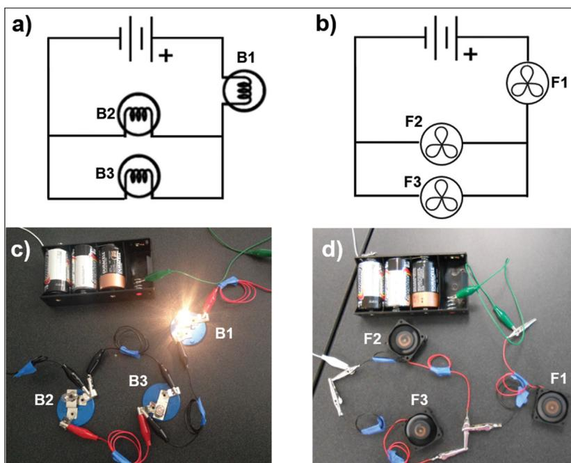
**Fig. 2.** Circuit diagrams for a combination bulb (a) and fan (b) circuits of two in parallel with one in series, as well as pictures of wired bulb (c) and fan (d) circuits. See a video of the fan experiment at *TPT Online* at [http://dx.doi.org/10.1119/1.4972490\\_2](http://dx.doi.org/10.1119/1.4972490_2).
