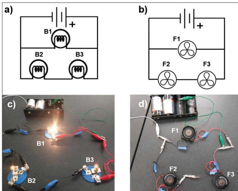
**Fig. 1.** Circuit diagrams for a combination bulb (a) and fan (b) circuits of two in series with one in parallel, as well as pictures of wired bulb (c) and fan (d) circuits. See a video of the fan experiment at *TPT Online* at [http://dx.doi.org/10.1119/1.4972490\\_1](http://dx.doi.org/10.1119/1.4972490_1).
