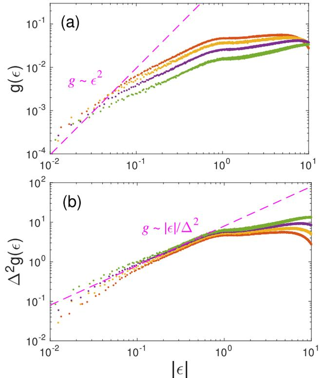
FIG. 4. (a) Density of states as a function of energy for different values of  $\Delta$ , as measured by our numeric simulations. From highest to lowest, the curves correspond to  $\Delta = 10, 12, 15$ , and  $20$ . The dashed line shows the 3D Coulomb gap equation. (b) When the DOS is plotted as  $\Delta^2 g(\varepsilon)$  versus energy, all the data collapses onto a single curve  $g(\varepsilon) \sim |\varepsilon|/\Delta^2$  within the energy range  $1/R_g \ll \varepsilon \ll 1$ .
