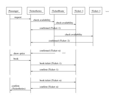
Figure 4: Sequence diagram to order a set of tickets.
